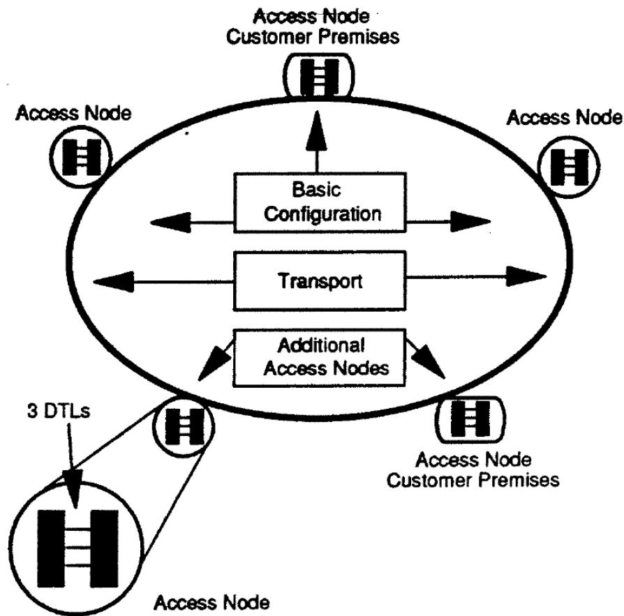
This configuration depicts an STN arrangement using the Basic Configuration equipped with DTL Volume Option 3 which includes three Access Nodes and three DTLs, plus two Additional Access Nodes.
