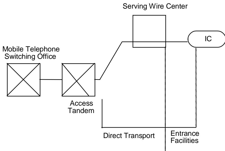
Cellular Mobile Carrier Interconnects with Local Exchange Carrier
