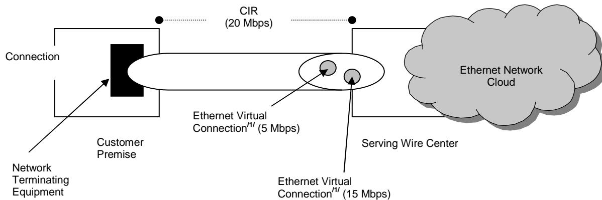
/1/ Ethernet Virtual Connections are used to establish a path for certain traffic between two customer locations, and do not have a charge associated with them. Each EVC must have a portion of the Committed Information Rate (CIR) service element assigned to it.
