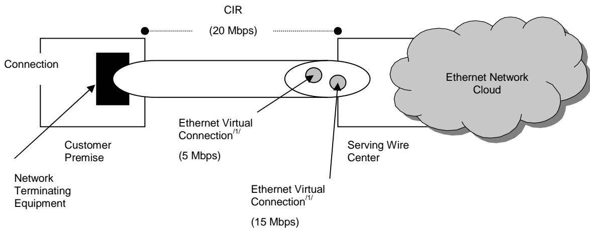
/1/ Ethernet Virtual Connections are used to establish a path for certain traffic between two customer locations, and do not have a charge associated with them. Each EVC must have a portion of the Committed Information Rate (CIR) service element assigned to it.
