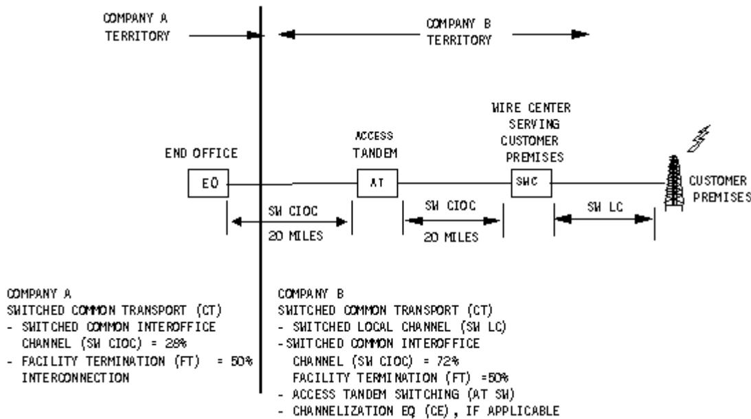
Assume 20 miles of Switched Common Transport (CT); **20 miles of Switched Dedicated Transport (DT)**; and 8,000 minutes of use. **Further**, assume a billing factor from NECA 4 of 28% for Company A and 72% for Company B.
